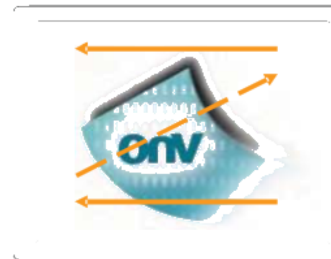
Fig. 2 Reverse scan (Pin19, RSV = High or VDD)
